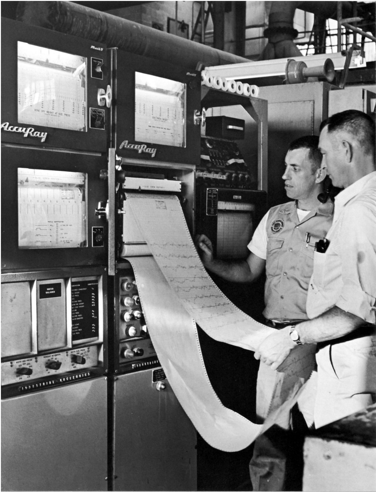
Paper machine operators reviewing cross machine direction profiles using the Series E recorder charts
