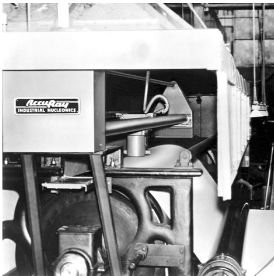
Figure 10 –Industrial Nucleonics scanning beta gauge at Champion, Lawrence MA, 1954
