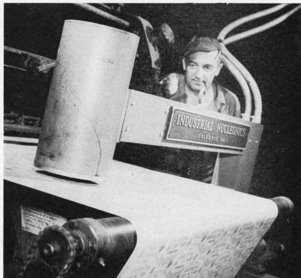
Radioactive isotope — strontium-90 — provides beta-rays that actuate gage for continuous measurement of unit weight and density as backing material passes through the abrasive coating machine at 350 fpm
